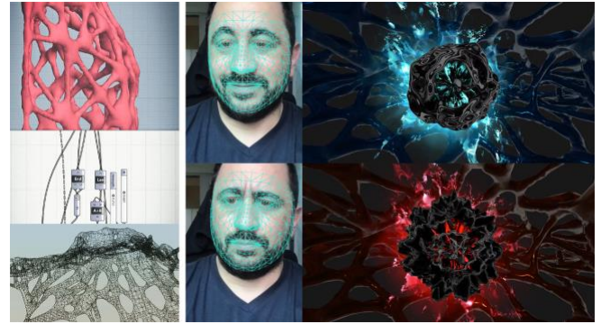
Fig. 2. Parametric modelling of the structure (left), facial expression tracking (middle), real-time visualization (right).
